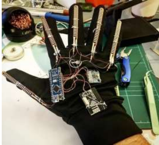
Fig I: Wireless Hand Motion Controlled Robotic Gripper Arm
